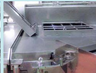
● Enclosed cover on material inlet
